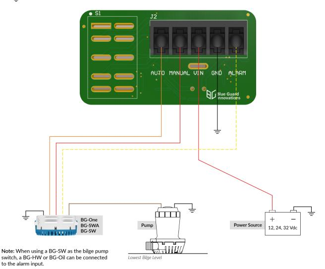
BG-CP-A with BGI Sensors | WIRE GUIDE | REV A www.bluebgi.com
