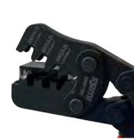
4. Place terminal into crimper at marked 16-14 AWG slot
