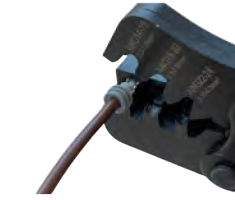
5. Place prepped wire into terminal and crimp
