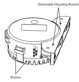
\*The BG-SW can also be mounted on the hull using three #8x0.75" 316 stainless steel screws. Mount the strainer irst, then attach the BG-SW into place.
