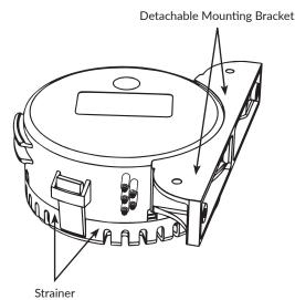
\*The BG-SWA can also be mounted on the hull using three #8x0.75" 316 stainless steel screws. Mount the strainer irst, then attach the BG-SWA into place.
